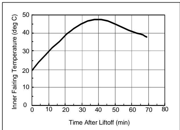
Figure 6-5. PM Inner Surface Temperature
